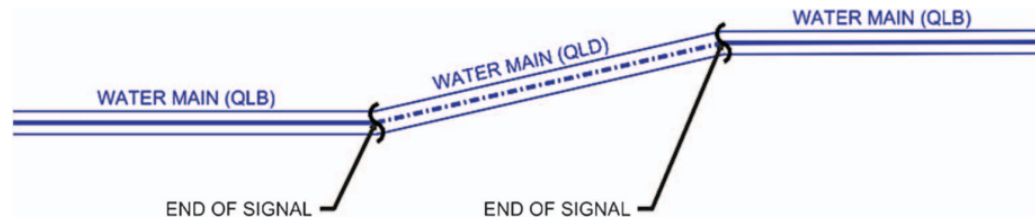
Figure 2-11. Portion of water main not continuously designated, requiring a separate utility segment at a more uncertain utility quality level.
